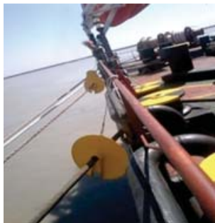
Figure 50. Anchored ship with rat guards
